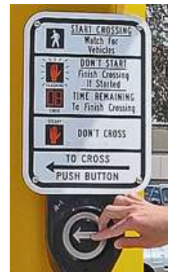
ACCESSIBLE PEDESTRIAN SIGNALS
